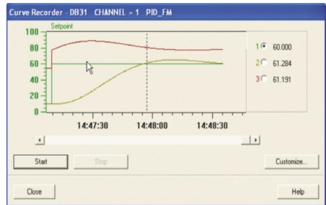
Controller optimization with the FM 355-2 temperature control module
