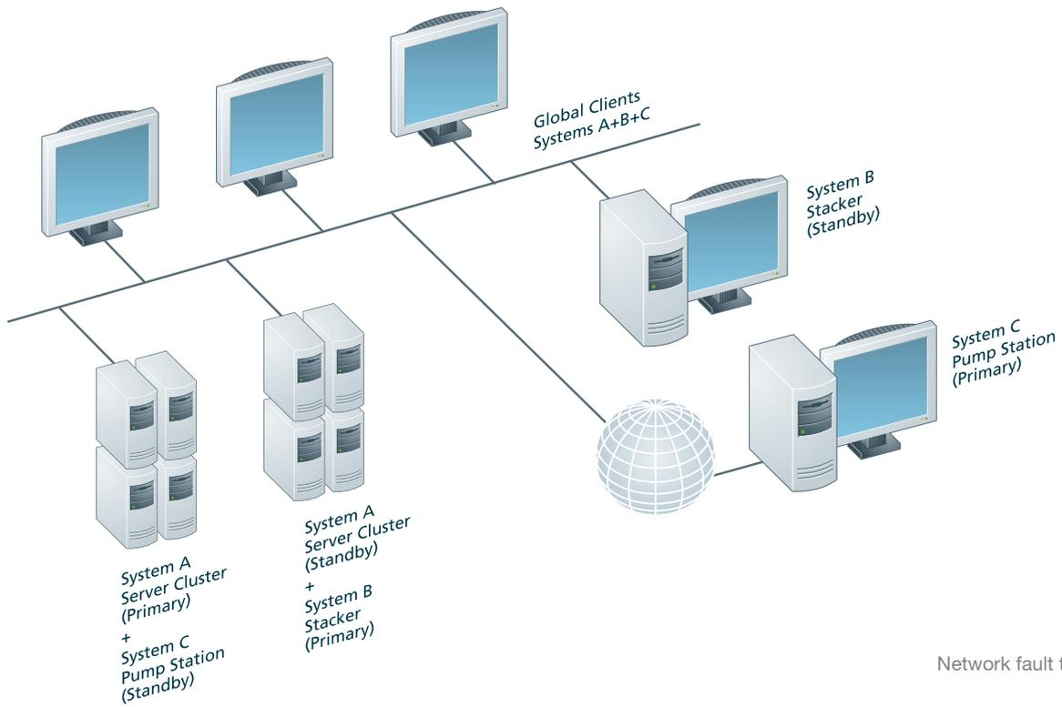
Network fault tolerance
