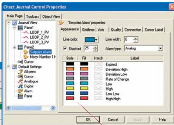
Alarm pens can represent different alarm states with colours or fill patterns.
