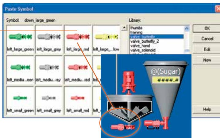
Symbols can change dynamically based on the state of a device. For example, you could assign two pump symbols to a device using different coloured symbols for running and stopped indications.
