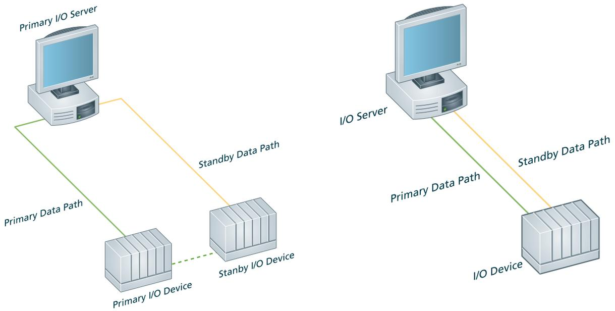
I/O device redundancy; data path redundancy
