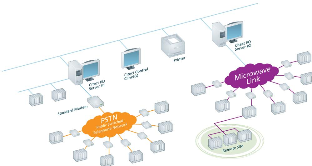
Remote Device Monitoring can be used in conjunction with up to 255 I/O servers to support applications with hundreds of thousands of points.
