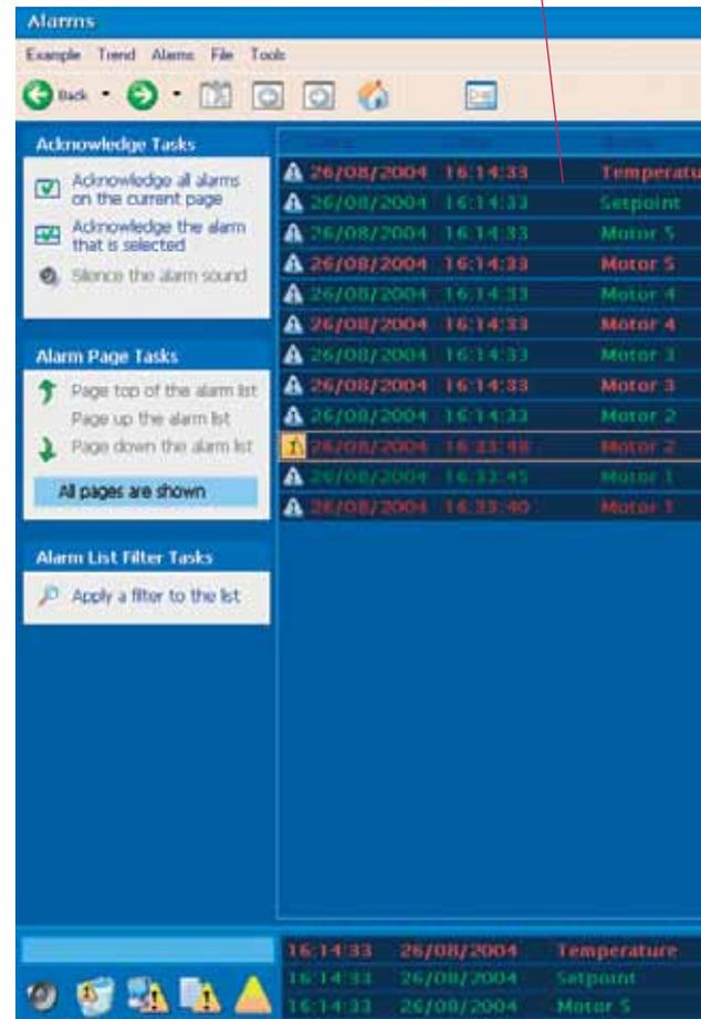
Flexible alarm formatting permits display of any related variable when the alarm is triggered.
