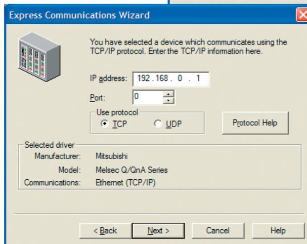
Select the manufacturer, model and communications method specific to the I/O device. Enter the address for the I/O device. It's that simple!
