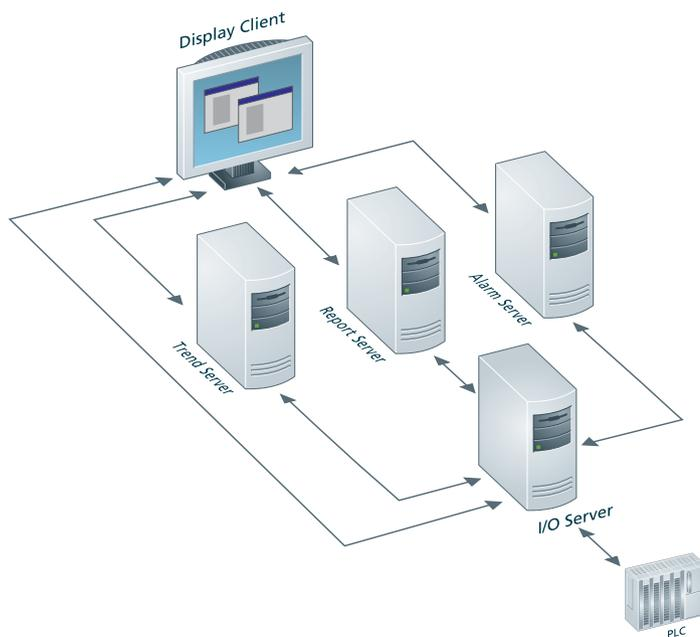
With the tags available, Vijeo Citect tasks can now be located to meet the requirements of the system. Often Vijeo Citect systems are built around a central pair of servers, each acting as the primary or standby server for all the Vijeo Citect tasks. This design will optimise its performance by executing each Vijeo Citect task individually.
